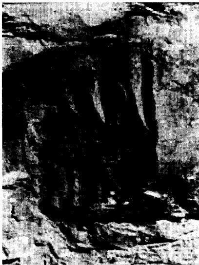
Fig. 3. A fracture cutting Lower Eocene chalk in the Shefela syncline. En échelon fringes occur on both the upper and lower sides of the parent joint. There is a clockwise rotation of the en échelon segments with respect to the parent joint in the upper fringe and a counterclockwise rotation in the lower one. Cracks in the two fringes differ considerably in shape. Scale bar is 10 cm.
